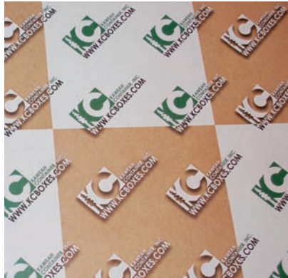
ON THE BACK OF THE PACKEXPO SAMPLES WAS THE COMPANY NAME, LOGO, WEB ADDRESS AND KRAFT DIGITALLY PRINTED ON MOTTLED WHITE LINER.
